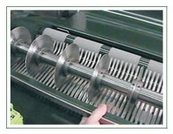
The screws must not be tight. The grate should be able to move up and down.
