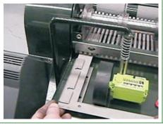
Position the guide to line up with the first blade. Set position. Use a straightedge to ensure accuracy.
