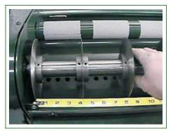
Carefully move blade assembly into position. Set blade positions and tighten screws.
