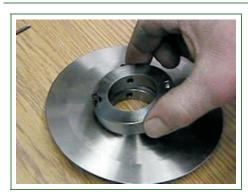
Line up the blade notches with the holes. Keep the set screw holes together.
