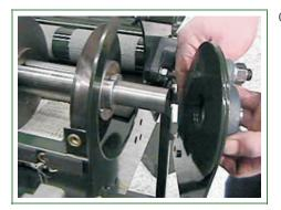
Carefully slide blade assembly off.
