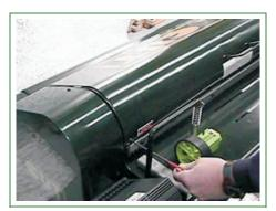
Remove the screws from the cover on the right side. Remove the screws from the cover on the left side.
