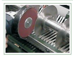
While the machine is running, using your angle grinder with 120grit to sharpen the blades. Sharpen both sides at about 15deg. The proper safety gear must be used while sharping!
