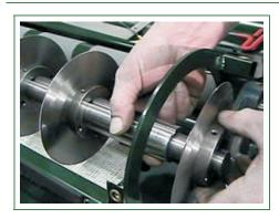
Loosen the blade and carefully remove the blade.
