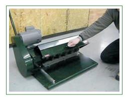
Remove the screws from the cover. Using the handle gently raise the cover.
