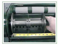
Loosen set screws. Carefully move blade assembly into position. Tighten screws.
