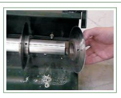
Loosen the set screws. Carefully slide the blade assembly off.
