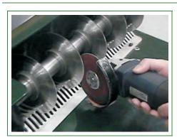
While the machine is running, using your angle grinder with 120grit. Sharpen both sides at about 15deg. The proper safety must be used while sharping!
