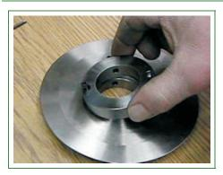
Line up the blade notches with the holes. Keep the set screws holes together.
