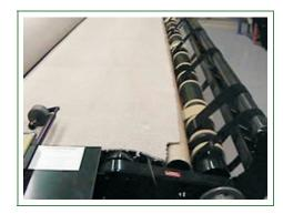
Position core. Set left FWD, Right REV. Advance carpet to middle of the core.
