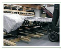
Use the forklift to lift the machine of the crate base from the broadside. Layout footpad strips flat side down. (only on some models)
