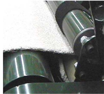
➤ While gently holding this Handle in place, press the Jog Button to continue the advancement of the carpet. You will only have to hold the Handle in place for 1 or 2 seconds at which time you will see the plates actually force the carpet around the core. Once you see the carpet is starting to wrap around the core, release the Handle to its original position.
