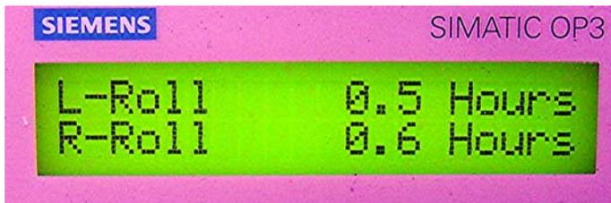
**Feature:** This screen shows the hours of motor run-time on both the left and right side rollers. You cannot change these values.
