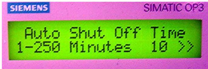
Feature: This screen allows you to set how long the machine will stay on before it automatically shuts off if it is not used. The factory setting is 10 minutes.
