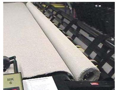
**IMPORTANT NOTE: IF YOU CONTINUE THE ROLL-UP PROCEDURE BY PRESSING THE JOG BUTTON INSTEAD OF THE FOOT SWITCH TAPE, THE MACHINE WILL NOT STOP AUTOMATICALLY AT YOUR PRE-SET LENGTH. BE SURE TO USE THE FOOT SWITCH TAPE AFTER YOU HAVE GOT THE CARPET STARTED SO THIS FUNCTION CAN PERFORM PROPERLY.**
