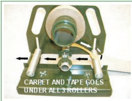
Carpet and tape goes under all 3 rollers
