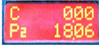
➤ For Example if you need to make an **18' 6"** cut, simply program the Pre-Set length in the **"PROCESS"** Pre-Set Screen to read **"18.06"**.
