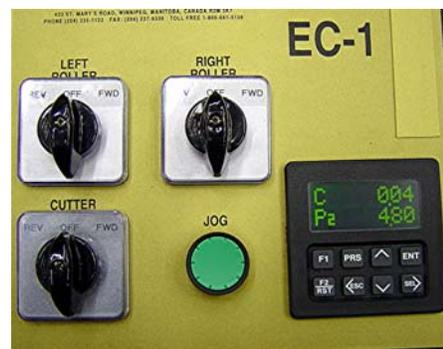
➤ Check that the Cutting Bar is working by pushing & holding the Cutter Switch to FWD. Since it is a Two-Way Cutter, you can make your next cut by pushing & holding the Cutter Switch to REV.
