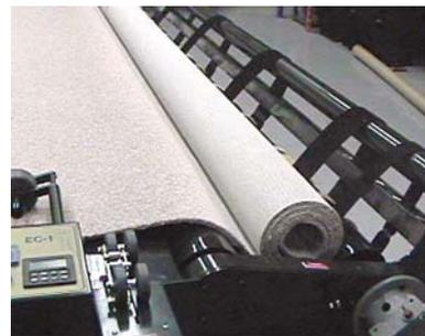
**IMPORTANT NOTE: IF YOU CONTINUE THE ROLL-UP PROCEDURE BY PRESSING THE JOG BUTTON INSTEAD OF THE FOOT CABLE, THE MACHINE WILL NOT STOP AUTOMATICALLY AT YOUR PRE-SET LENGTH. BE SURE TO USE THE FOOT CABLE AFTER YOU HAVE STARTED THE CARPET SO THIS FUNCTION CAN PERFORM PROPERLY.**
